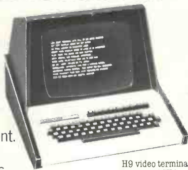
H9 video terminal, with 87 ASCII keys.
